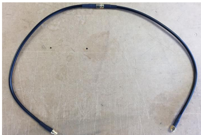
Connected LMR-195 cable
