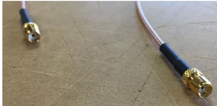
RG 316 Cable with SMA Female Jack – A5530H and A5530C's Pigtail
