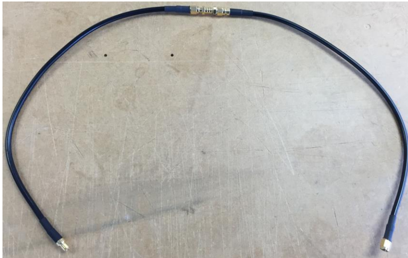
LMR-195 Cable connected using an adapter
